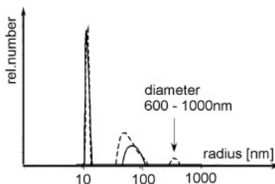
**Fig.1:** Dynamic light scattering on a ferrofluid sample, sampling time 3s (solid lines) and 1h (dashed lines).
