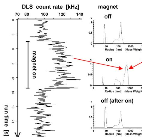
Additional samples were prepared for the electron microscopy in the magnetic field. Micrometer sized chains were observed. The chain length increased with the field strength. After removal of the field the chains disintegrated within the resolution (2 s) of the time resolved dynamic light scattering experiments.
