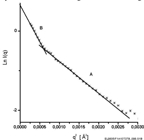
**Fig.2:** The Guinier representation of F<sub>1</sub>ATPase after 90 min azide inhibition indicates the formation of a larger species ( $R_g = 71.24 \pm 1.05 \text{ \AA}$ ,  $\Delta t = 1 \text{ min}$ ) by the linear range B in the USAX region ( $q = 0.016\text{-}0.025 \text{ \AA}^{-1}$ ).
