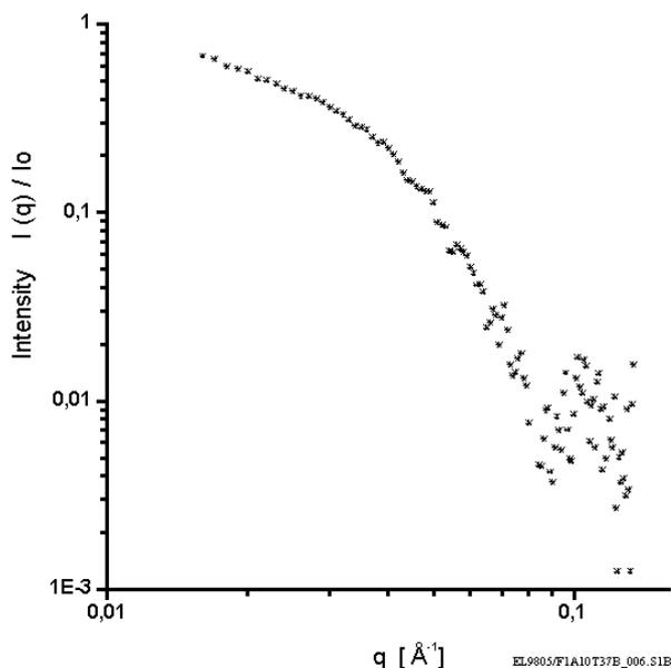
**Fig.2:** X-ray small angle scattering of F<sub>1</sub>ATPase during azide inhibition obtained during a 10 s exposure. The spectrum is a frame of a structural film of 128 pictures after rapid mixing of native enzyme and azide by a stopped flow device (5g/l protein, 10mM N<sub>3</sub>).
